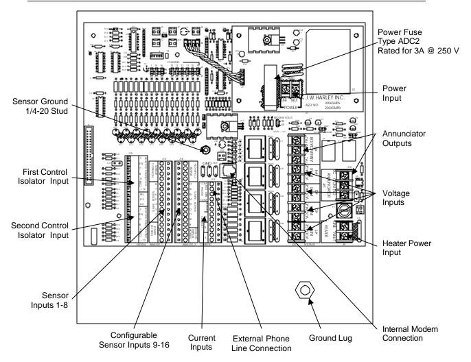
Figure 3-4: Fuse, Input Terminals, and Ground Locations
